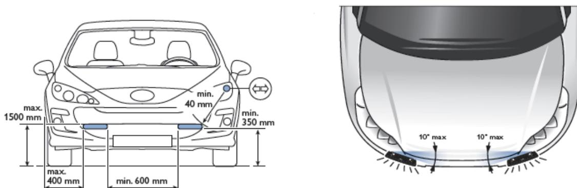
Make sure that the installation position of the lamps conforms to the diagram above. To adjust the lamps to the shape of the bumper you can lean the lamp and modify the horizontal tilting angle up to 10°.
